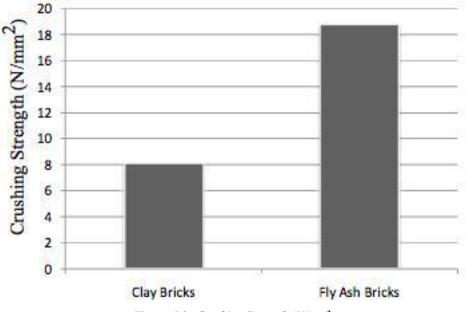
Figure: 5.2. Crushing Strength (N/mm<sup>2</sup>)
