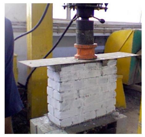
4.1 Prism Test for Fly Ash Bricks
