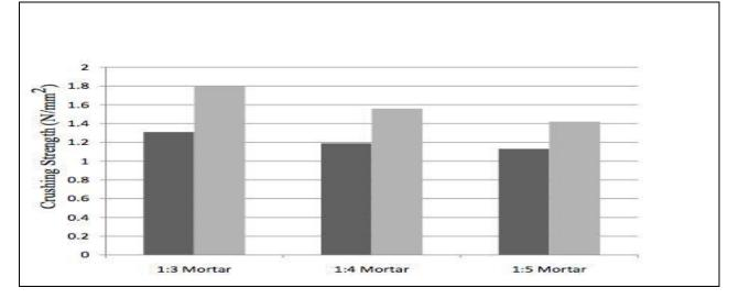
Figure: 5.3. Crushing Strength By Prisms (N/mm<sup>2</sup>)
