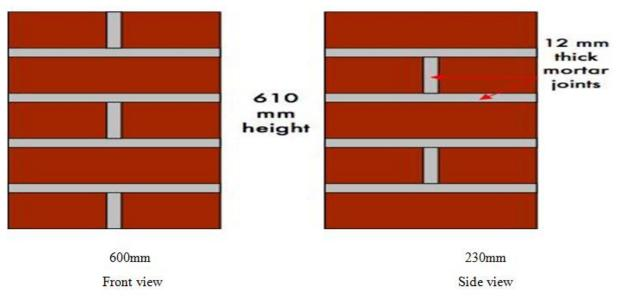
Figure 4.1: Typical Size Of Prisms For Compressive Strength Test
