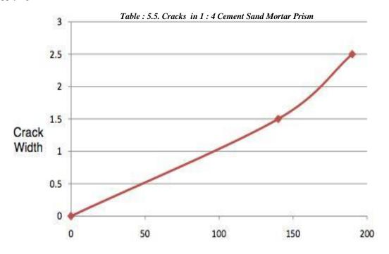
In prism testing of 1:4 cement sand mortar maximum width of crack appeared to be 1.5 mm and average width of crack was 1 mm on applying load of 140 KN. On again applying load crack were measured with the maximum width of 2.5 mm and average crack width of 1.5 mm by applying load of 190 KN.Prism of 1:4 cement sand mortar failed on applying load of 264 KN.
