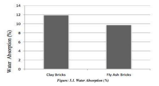
As per the above table, the average absorbed moisture content of clay bricks is found to be 11.93% and for fly ash bricks is found to be 9.77%. Thus there is net 18.10% decrease in moisture absorbed for fly ash bricks as a part to clay bricks.
